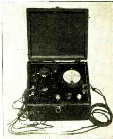
The completed Tester. The test prods and wire shown are standard equipment in all shops and service men's kits. The carrying case may be arranged to tilt, if desired.
